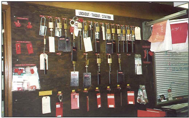
This is Tacoma's lock-out panel board. The padlocks on this board are shift locks which are used when a shift change occurs before maintenance work is completed. The other tools are special devices to permit locking out different types of switches or valves. Tags are always used to indicate why the device is locked out. Tag-out tags are used when it is not possible to install a lock. Each worker's personal lock is marked or tagged to identify the lock's owner
